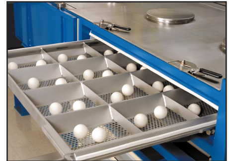
Balls reduce blinding of near-size material.
